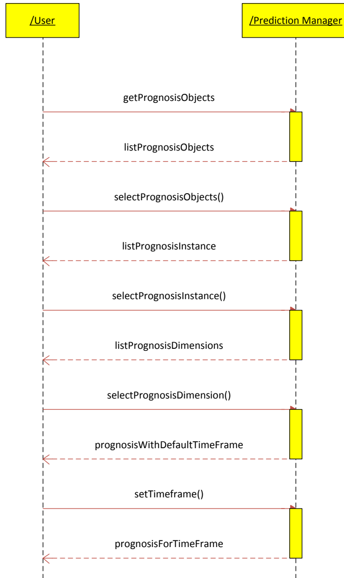
Figure 45: Overview of the user interaction with the Prediction Manager for requesting a specific prognosis
